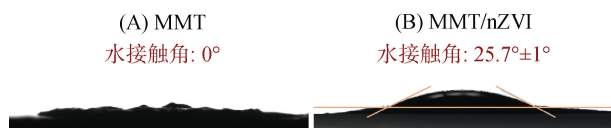
图3 MMT(A)和MMT/nZVI(B)的水接触角 Fig. 3 Water contact angles of MMT(A) and MMT/nZVI(B)
