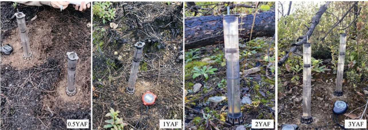
图 3 林火迹地不同恢复年限水分入渗试验 Fig. 3 Water infiltration experiments in forest fire areas with different restoration years
