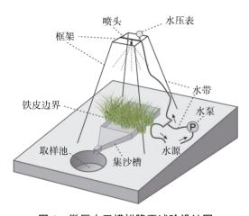
图 1 微区人工模拟降雨试验设计图 Fig. 1 Design scheme of artificial rainfall in micro-plot
